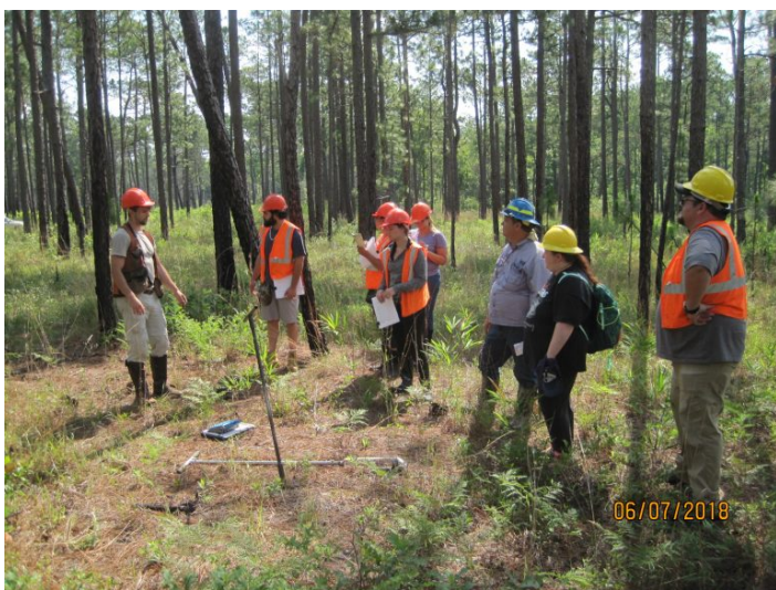
The group used soil augers to practice delineating wetland boundaries. Photo by Randy Fowler, USFS.
